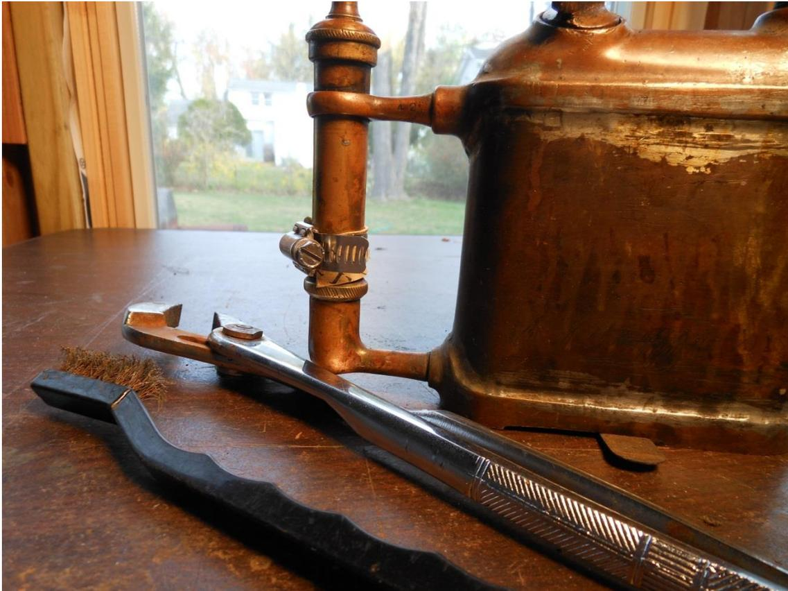
Always remember: The goal is to leave NO tool marks. Usually they have enough to start with. If you have to strain to remove a part, STOP. You run the risk of damaging the part. Go to the backup plans of Liquid Wrench and heat. When applying heat, make sure you keep it localized on the part you are working with. You do not want to melt the solder on other parts of the torch.
